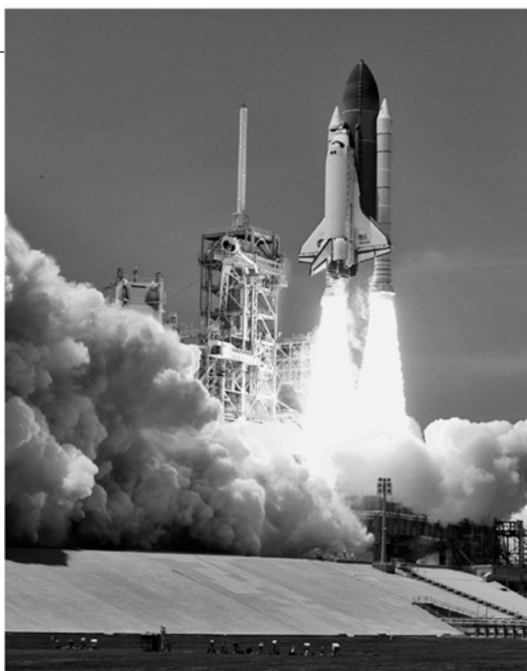
FIG. 1.1. A space shuttle launch: chemical potential energy (liquid hydrogen and liquid oxygen fuel) is converted into the kinetic energy of the speeding rocket, in order to overcome the gravitational potential energy of the Earth. Photo courtesy of NASA.
